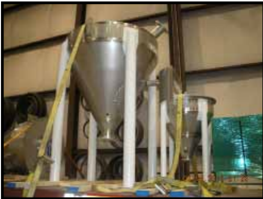
Scale Hoppers 304-2B Stainless Steel Product Contact Carbon Steel Non-Product Contact 36-Grit Polished Product Contact Welds External Welds Cleaned of Smoke
