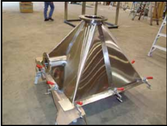
STE3x40H Filter/Receiver 304-#4 Stainless Steel Product Contact 304-#4 Stainless Steel Gas & External Contact 180-Grit Polished Welds on Product Contact 180-Grit Polished Welds on External Seams
