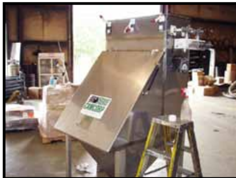
Model BD40 Bag Dump Station 304-2B Stainless Steel Product Contact Carbon Steel Gas & External Contact Internal Welds Ground Smooth External Welds Cleaned of Smoke
