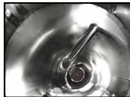
Model 3PRT10 Filter/Receiver Hopper 316-2B Stainless Steel Product Contact 120-Grit Polished Welds on Product Contact Interior & Exterior Surfaces Electropolished
