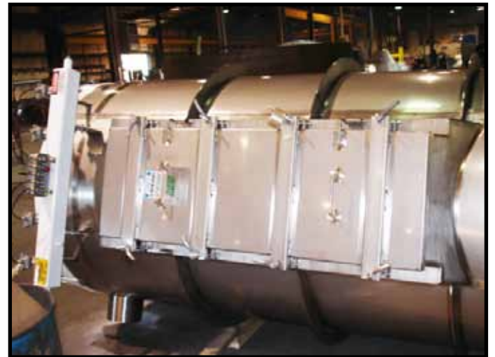
Model 8PRB24 Filter/Receiver 304-2B Stainless Steel Product Contact Carbon Steel Gas & External Contact 80-Grit Polished Welds on Product Contact External Welds Cleaned of Smoke
