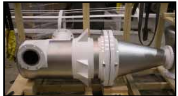
Model HE19 Cyclone 304-2B Stainless Steel Product Contact Carbon Steel External Contact 36-Grit Polished Product Contact Welds External Welds Cleaned of Smoke
