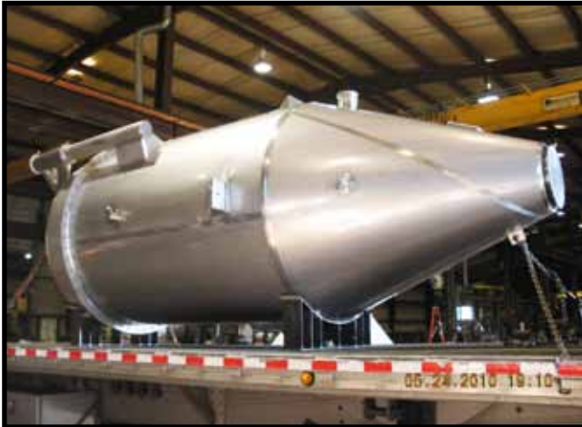
Model 6PRT31 Insulated Filter/Receiver 316L-2B Stainless Steel Product Contact 304-2B Stainless Steel Gas Contact 304 Stainless Steel External Surfaces 180-Grit Polished Welds on Product Contact 36-Grit Ground Welds on External Skin
